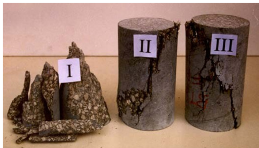
Figure 6: State of the test-tubes after break (simple compression).
