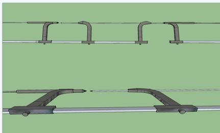
**Figure 2:** Suggested conception of a tunnel aimer that keeps the femoral and tibial tunnel in one axis. All four movable aimers slide on metallic band to keep all aimers in one line and insure that the guide wires pass from tibia to femur or from femur to tibia in one line.
