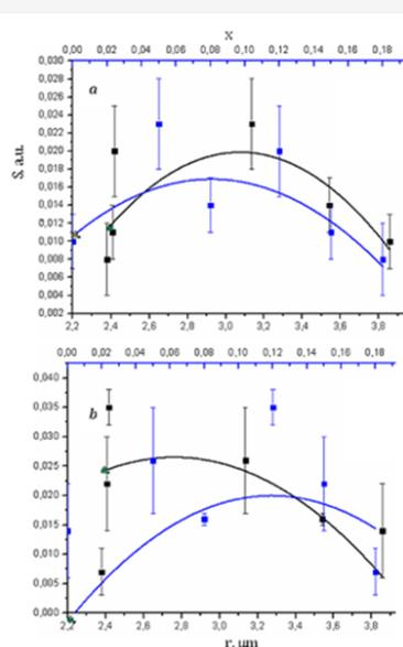
**Figure 1:** Dependences of the density of the blackening ( $S$ ) of the X-ray film on the composition and particle size of  $\text{La}_{1-x}\text{Gd}_x\text{TaO}_4$ .  $I = 40$  mA,  $t = 120$  mc. a:  $U = 40$  kV; b:  $U = 52$  kV.
